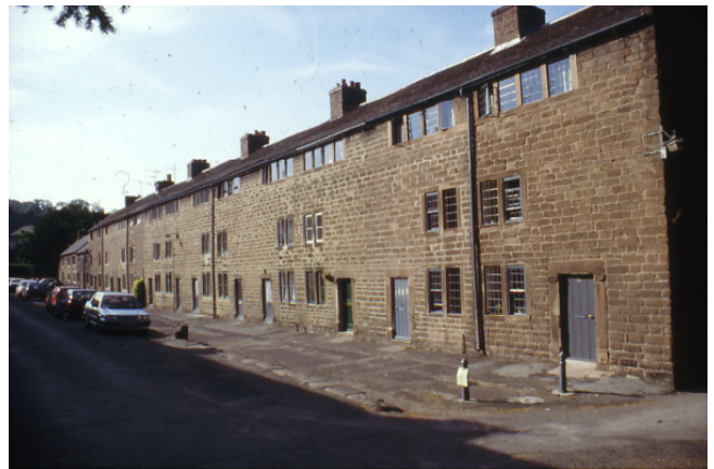
North Street, Cromford, some of the first houses built for his workers by Richard Arkwright. The rooms on the top floor with long-light windows would have been used for weaving or framework knitting.
